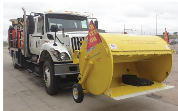
Figure 2: Road debris remover instrument used in the U.S.
