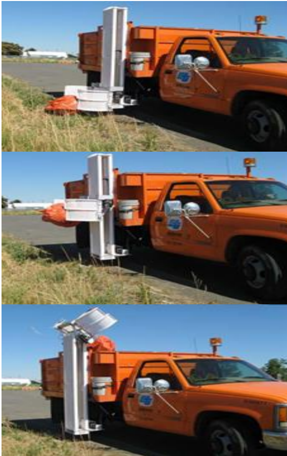
Figure 3: Roadside trash remover used by the U.S. Caltrans
