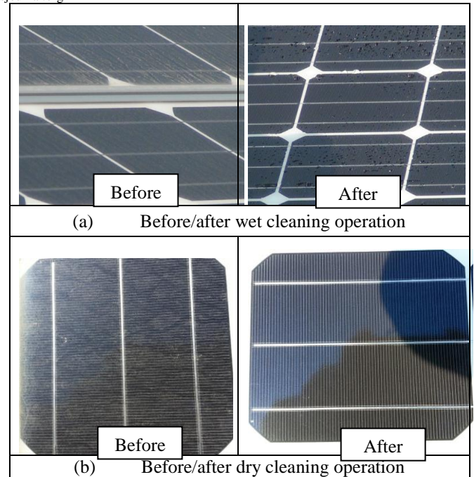
Figure 3: Result of operation of PV panel cleaning system
