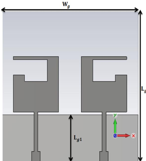
Figure 5: Compact MIMO antenna
