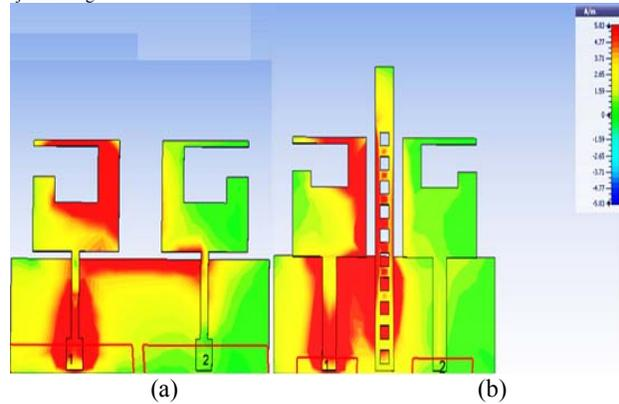
**Figure 15:** Surface current (a) without parasitic element (b) with parasitic element
