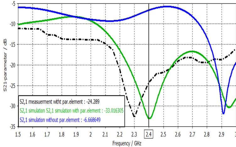
Figure 17: Simulated and measured of S<sub>21</sub>-parameter
