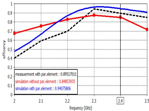
Figure 20: Simulation and measured efficiency values with/without parasitic element
