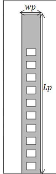
Figure 9:Geometric shape of the proposed parasitic element
