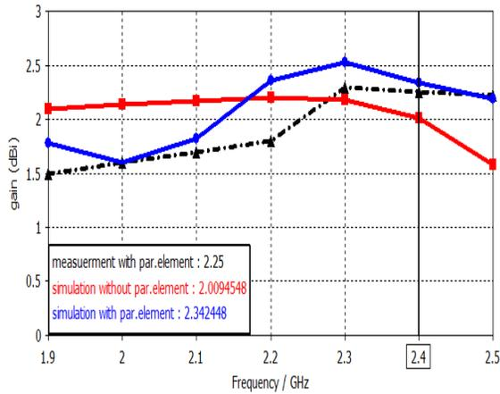
Figure 19: Simulated and measured gain values
