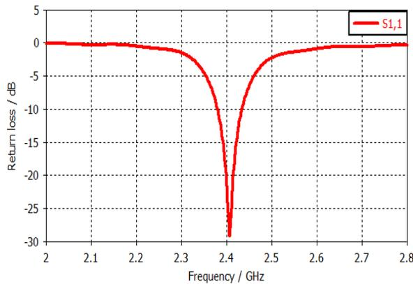
Figure 2: Return loss plot of the single rectangular patch antenna
