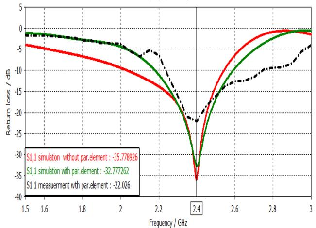
**Figure 16:** Simulated and measured  $S_{11}$  parameter
