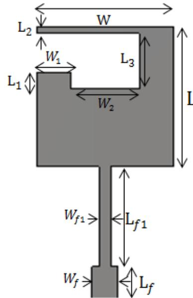
Figure 3: The optimized slotted patch
