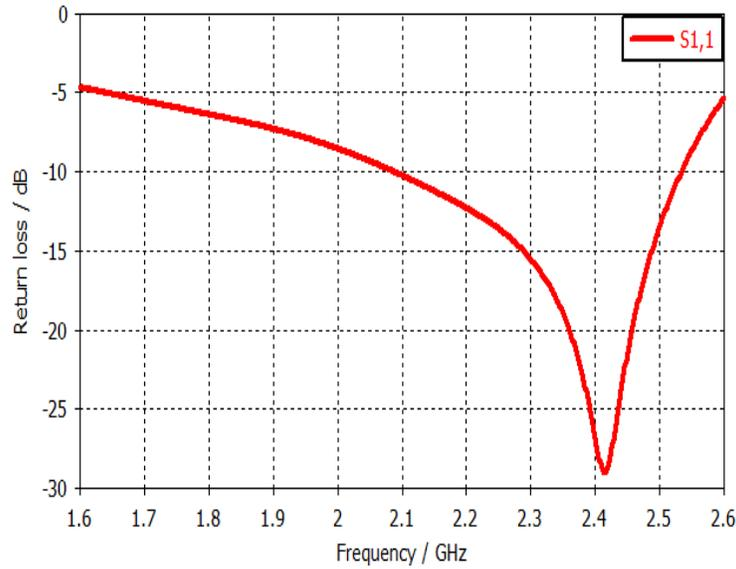
Figure 4: Return loss plot of the optimized slotted patch antenna
