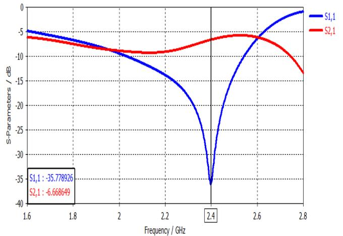
Figure 6: S-parameter simulation result of MIMO antenna
