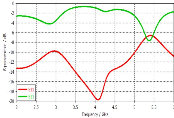
**Figure 11:** S-parameter simulation results of parasitic element
