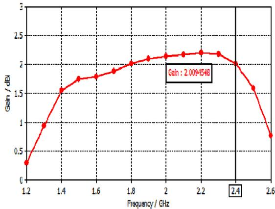
Figure 7: Total gain plot vs. frequency of MIMO antenna.
