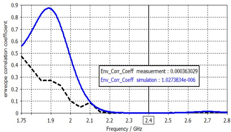
Figure 18: Simulated and measured results of envelope correlation coefficient
