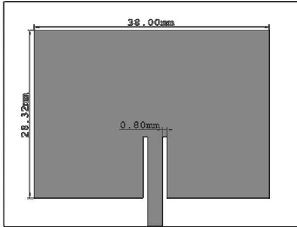
Figure 1: The single rectangular patch antenna
