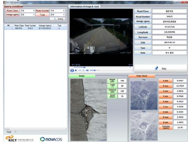
Fig 5: Query system for Pothole 2D DB
