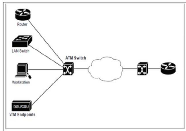
Fig 2: ATM network example
