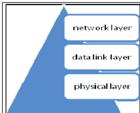
Fig 1: ATM Architecture layers
