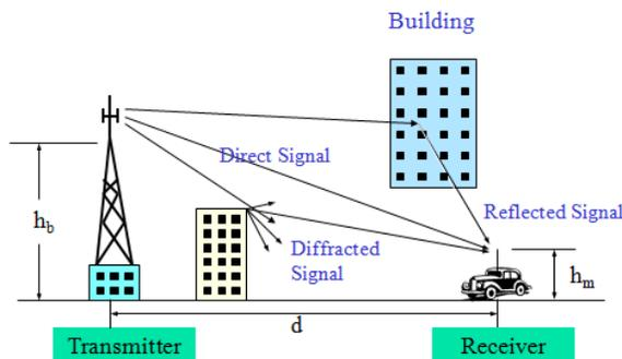
Fig 2: Some radio propagation mechanisms [18]
