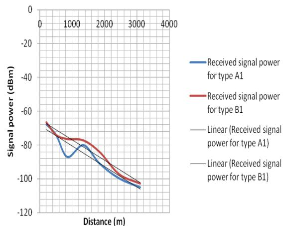
**Fig 5:** Graphs of received signal power against distance for type A and B networks in scenario 1
