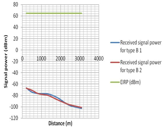
**Fig 4:** Graphs of received signal power and EIRP against distance for type B network for the two scenarios.
