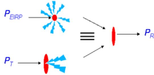
**Fig 1:** Illustration of the power transmitted from the transmitter to reception at the receiver
