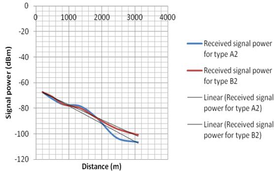
**Fig 6:** Graphs of received signal power against distance for type A and B networks in scenario 2
