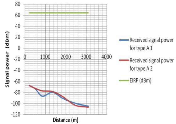
**Fig 3:** Graphs of received signal power and EIRP against distance for type A network for the two scenarios
