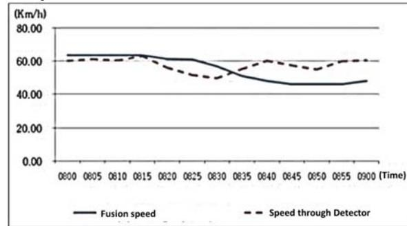
Fig 7: Comparison between Fusion Speed and ITS Speed Detector in Rural Area
