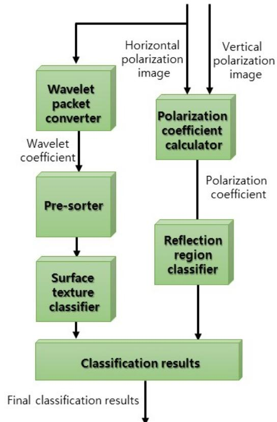
Fig 2: Road surface condition recognition process
