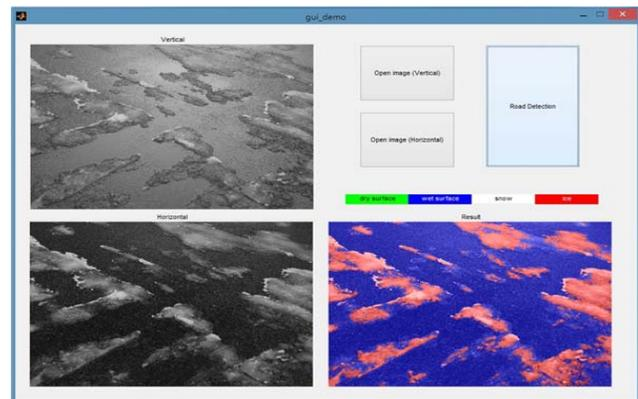
Fig 6: Initial screen of road surface recognition system
