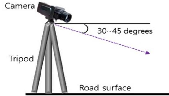
Fig 1: Road surface image acquisition method
