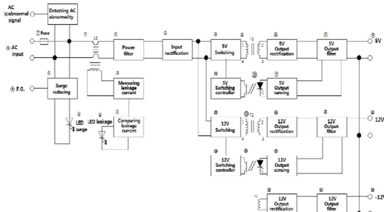
Fig 5: Block diagram of circuit for detecting leakage current and output voltage stabilization
