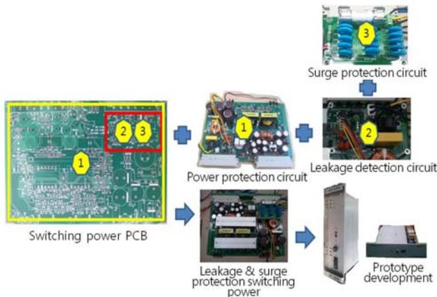
Fig 7: Power supply module with built-in leakage detection circuit
