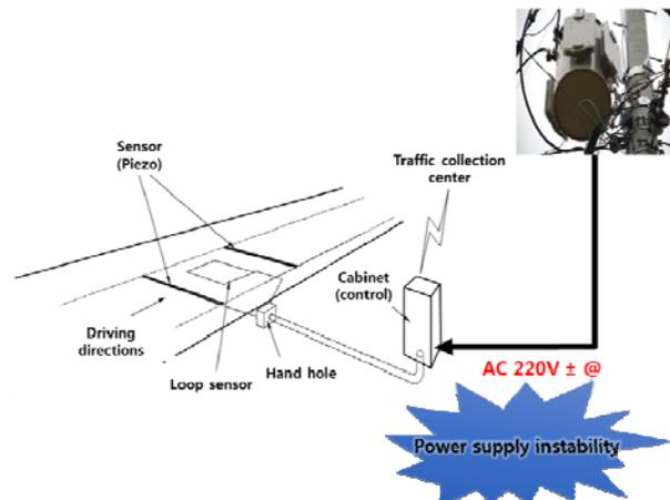
**Fig 1:** Common installation method of RSE
