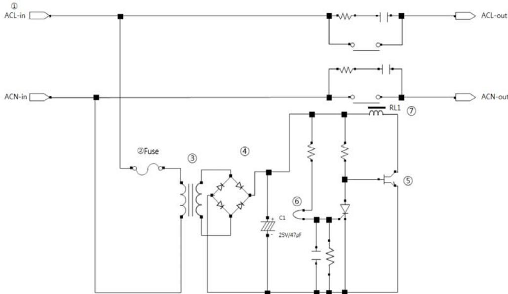
Fig 6: Power-off and recovery methods of controller from external noise
