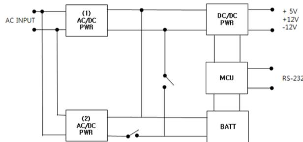
Fig 4: Dual power converter
