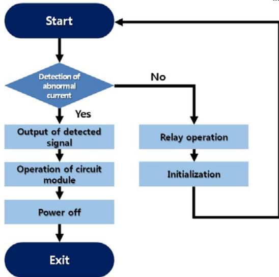
Fig 3: Noise detection and response procedures
