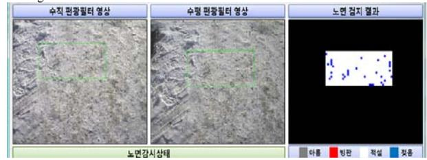
**Fig 15:** Snowy road surface detection screen
