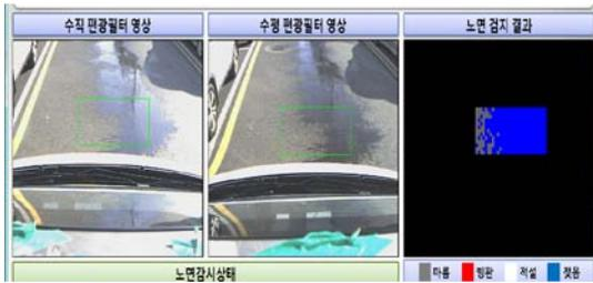
**Fig 12:** Wet road surface detection (Screen capture, driving speed: 0km/h)
