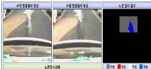
**Fig 13:** Wet road surface detection (Screen capture, driving speed: 50km/h)
