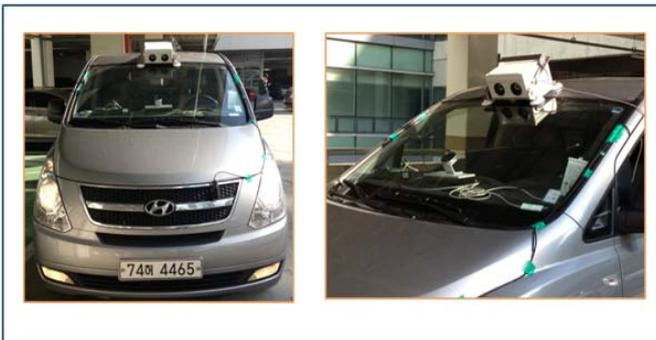
Fig 2: Mobile road surface condition detection system
