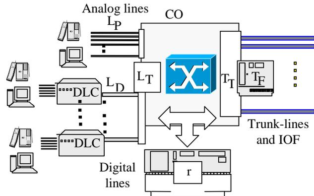
**Fig 2:** Technology-specific central office (CO) parameters that can be engineered to meet customer demand and for optimal revenue earning. (DLC: Digital loop carrier;  $L_P$ : Number of analog lines;  $L_D$ : Number of digital lines;  $T_T$ : Trunk terminations;  $L_T$ : Line terminations;  $T_F$ : Trunk facility; and,  $r$ : Call-processing capacity)
