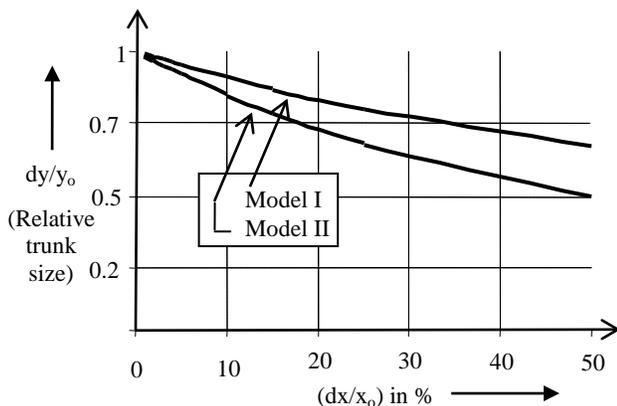
**Fig 3:** Fractional changes in x DSL growth versus trunk-size at the incumbent local exchange carrier (ILEC) CO: The cause-effect inverse proportion relation conforms to the proposed canonical Model I with  $\Gamma = 1$  and Model II with  $\Gamma = 1.75$ .
