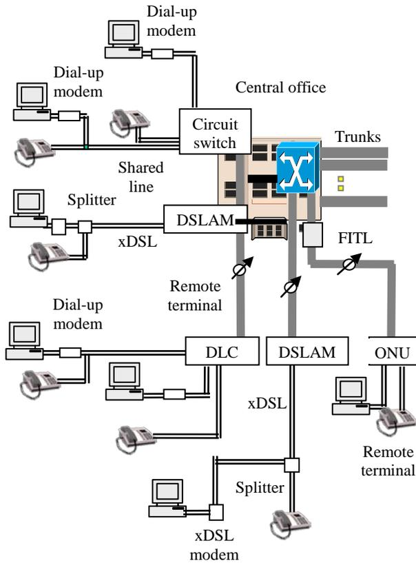
**Fig 1:** Typical telephone and data access methods at a local switching office (CO/RT) level. (DLC: Digital loop carrier; DSLAM: DSL access modem; FITL: Fiber-in-the-loop; ONU: Optical network unit)
