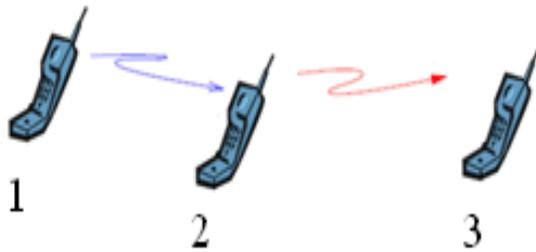
Fig 7: Cooperative system model with single relay [8]
