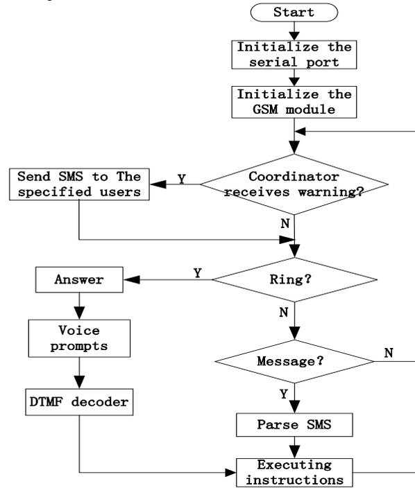
Fig 6: The control program's flow chart of GSM module
