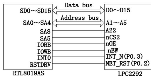
Fig 7: The connection diagram of RTL8019AS and LPC2292
