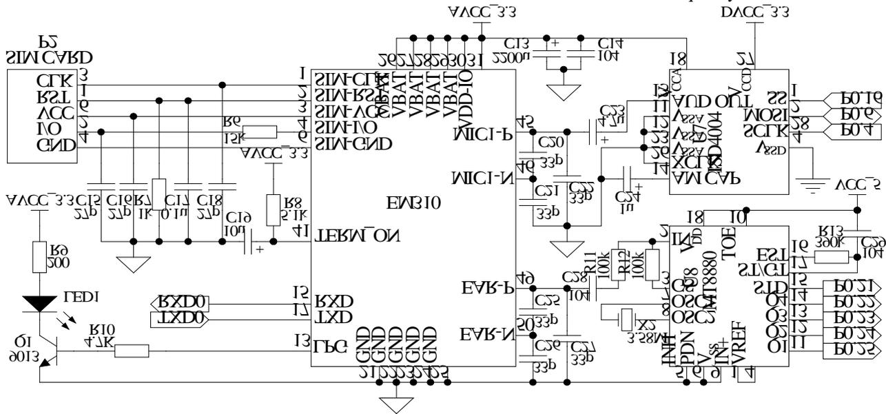
Fig 3: The main interface circuit of EM310 and LPC2292
