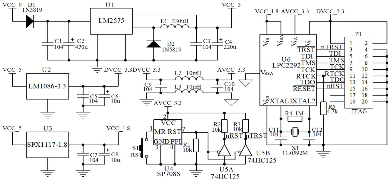
Fig 2: LPC2292 minimum system circuit
