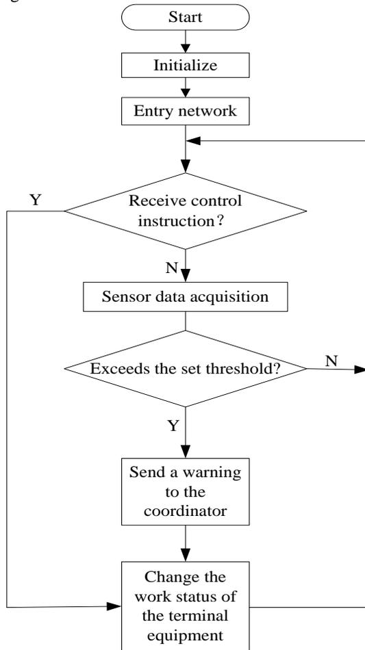
Fig 5: The program's flow chart of CC2530 MCU
