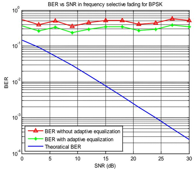
Figure 7: BER vs SNR in frequency selective fading for BPSK
