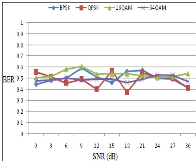
Figure 6: BER vs SNR in frequency selective fading without equalizer
