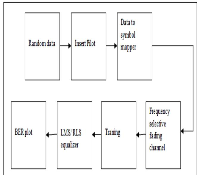
**Figure 4:** System model with adaptive equalizer
