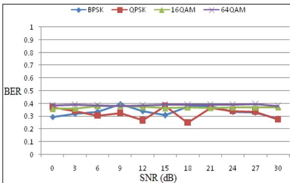
**Figure11:** BER vs SNR with adaptive equalizer
