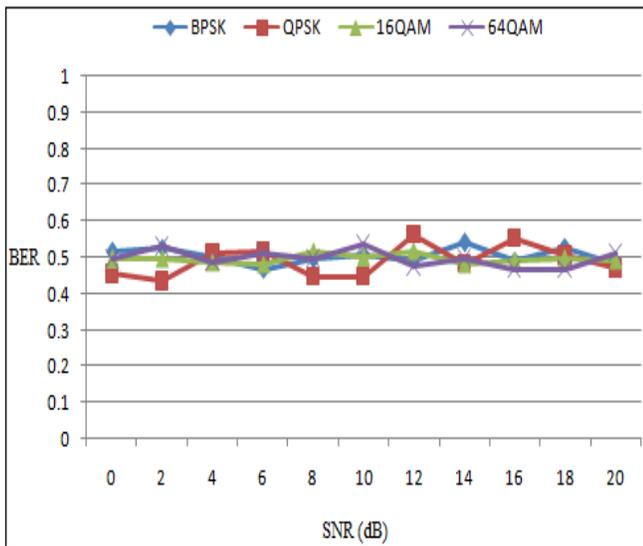
**Figure 2:** BER vs SNR in flat fading without channel estimation
