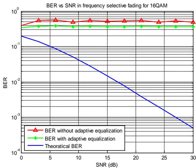
**Figure 9:** BER vs SNR in frequency selective fading for 16QAM
