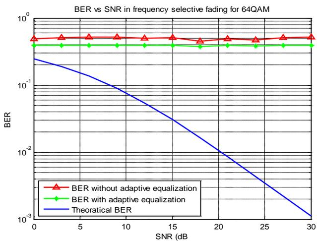
**Figure 10:** BER vs SNR in frequency selective fading for 64QAM
