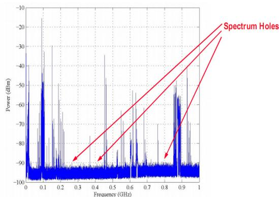
Spectrum measurement across the 900 kHz –1 GHz band (Lawrence, KS, USA)
