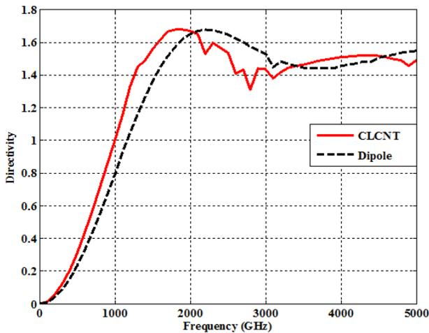
Fig 10: Directivity of CLCNT and SWCNT dipole antennas.
