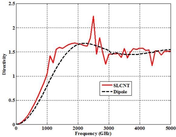
**Fig 4:** Directivity of SLCNT and SWCNT dipole antennas.
