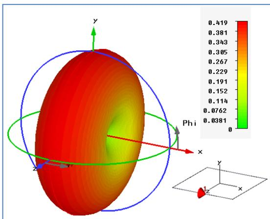
**Fig 6:** Radiation pattern for SLCNT antenna at  $f_{r1} = 586$  GHz.
