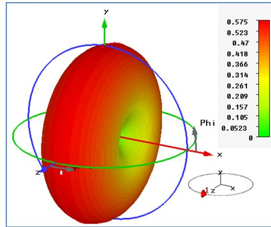
Fig 12: Radiation pattern for CLCNT antenna at  $f_r = 703$  GHz.
