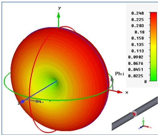
**Fig 5:** Radiation pattern for SWCNT dipole antenna at  $f_{r1} = 851$  GHz.
