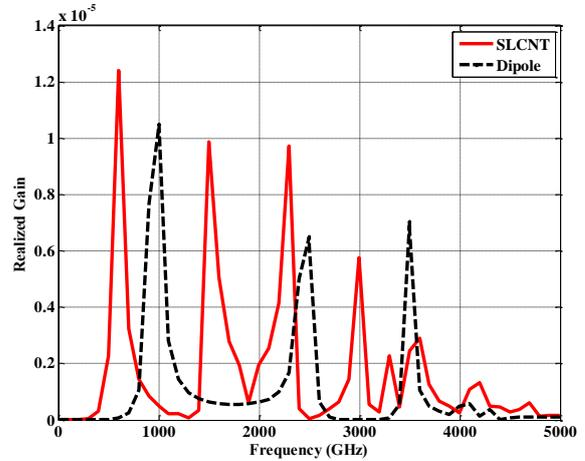
**Fig 7:** Realized gain of SLCNT and SWCNT dipole antennas.
