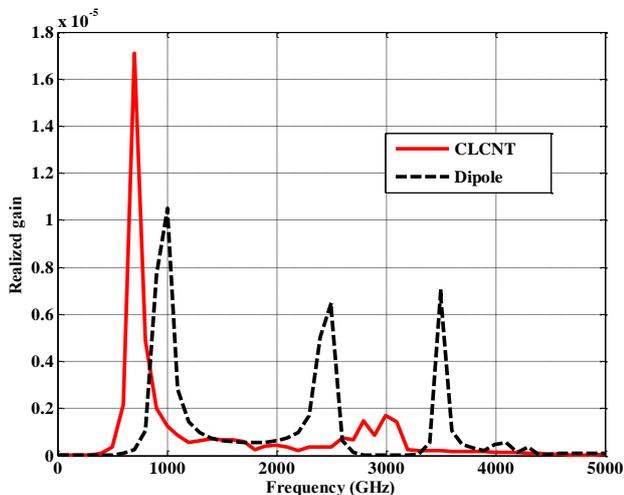
Fig 11: Realized gain of CLCNT and SWCNT dipole antennas.
