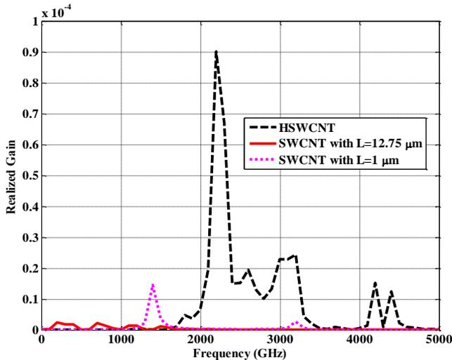
**Fig 16:** Realized gain versus frequency of HSWCNT antenna and SWCNT antenna with  $L = 12.57$  and  $1 \mu\text{m}$ .
