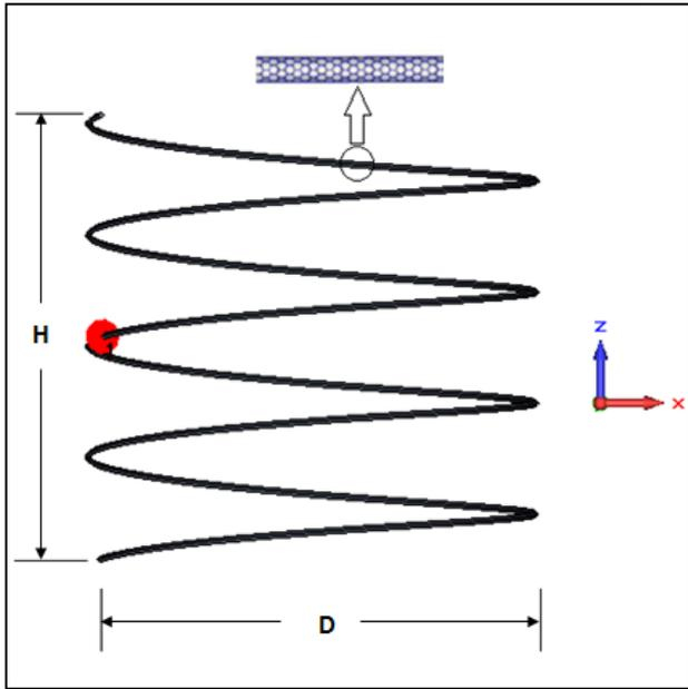
Fig 13: Geometry representation of the HSWCNT antenna.
