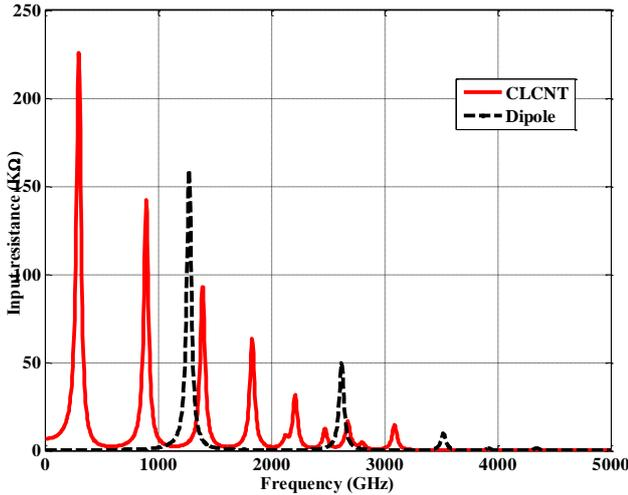
Fig 9: Input resistance of SLCNT and SWCNT dipole antennas.
