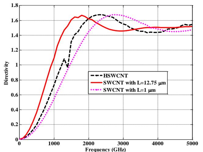
Fig 15: Directivity versus frequency of HSWCNT antenna and SWCNT antenna with  $L = 12.57$  and  $1 \mu m$ .
