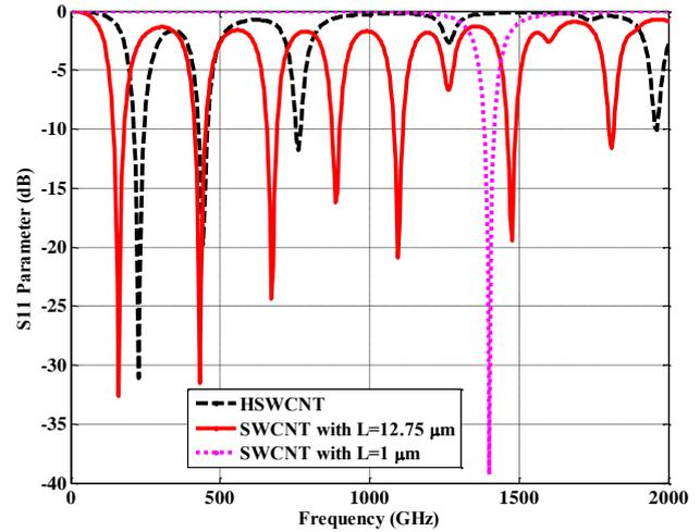
Fig 14: S<sub>11</sub> parameter of HSWCNT antenna and SWCNT antenna with  $L=12.57$  and  $1 \mu m$ .
