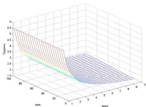
**Figure 5:** Total sensing time versus  $\beta$  and  $\alpha$ .
