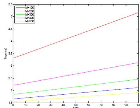
Figure 3: Total sensing time versus  $\beta$  for different number of antennas.
