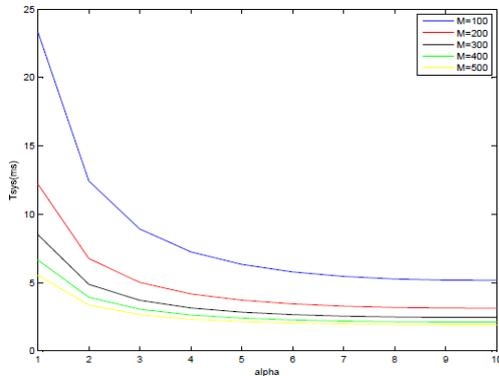
**Figure 4:** Total sensing time versus  $\alpha$  for different number of antenna.
